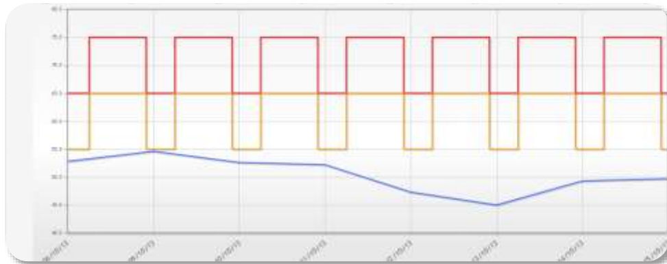
Figure 17: LAeq time history with Red and Orange thresholds
